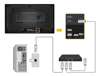
Connect the LAN cable between the [LAN] port on the product and the [LAN] port on your PC.
